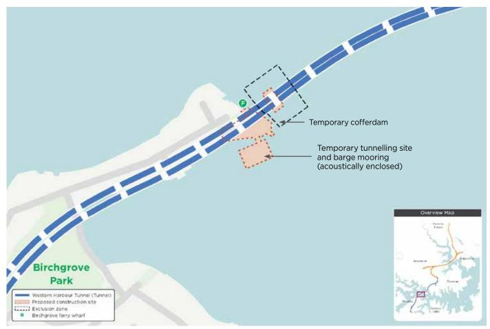
Temporary tunnelling site to support tunnelling under the Birchgrove peninsula and into the immersed tube transition structure for the Sydney Harbour crossing.
